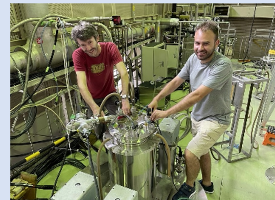
Left : Assoc. Prof. BADEL Right : Mr. VIALLE With a Test module for High Tc Superconductor Coil
